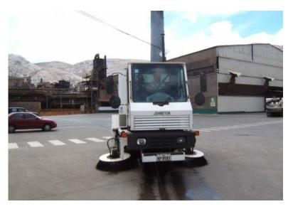
Once paved the roadways are subject to mechanical and manual cleaning 24 hours a day to ensure that the trucks and plant vehicles do not create any dust clouds. Total investment in the fleet of road sweepers is US \$ ~ 800 k.
