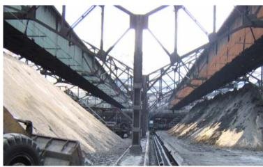
Fugitives from the fusion beds in both the copper and lead circuits have a new work regime designed to minimize the dust emissions by spraying a fine water mist onto the beds.
